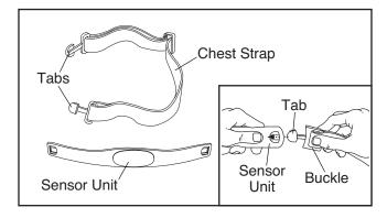
Next, wrap the chest pulse sensor around your chest and attach the other end of the chest strap to the sensor unit. Adjust the length of the chest strap, if necessary. The chest pulse
